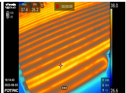
Thermal: radiant flooring at 2nd floor en-suite bathroom. Working at time of inspection
